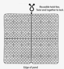
Secure overlapping edges of each Netfloat mat in the centre using the twist ties.
