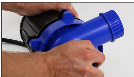
Step 10: Re-fit the impeller housing. This can be positioned at multiple angles.
