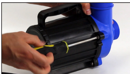
Step 12: Re-fit all four screws around the impeller housing and tighten up.
