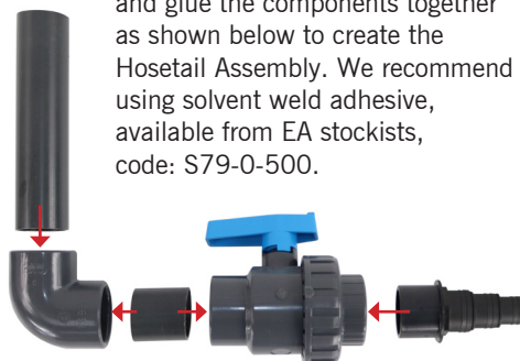
Figure 7.1. Hosetail assembly
